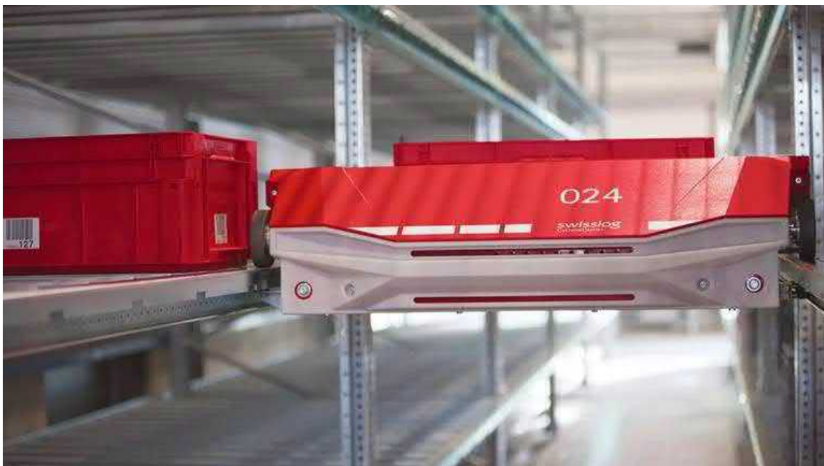
CycloneCarrier: Dynamic shuttle storage and retrieval system
